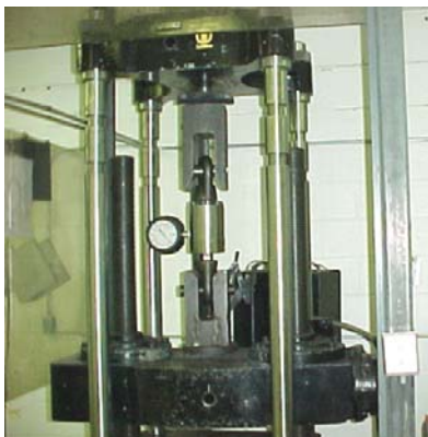
WS-10 Crane Scale on the test fixture.
